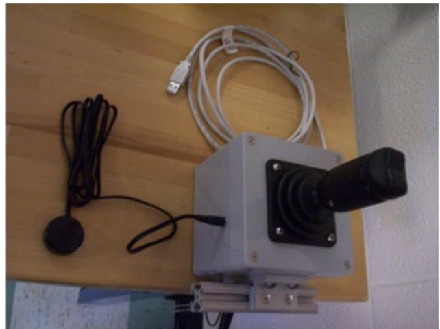
Fig. 14.16. Joystick in Encasement with Attached Optional Head Switch.
